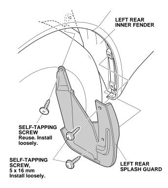
10. Secure the left rear splash guard to the rear bumper with a loosely-installed 5 x 20 mm self-tapping screw.
