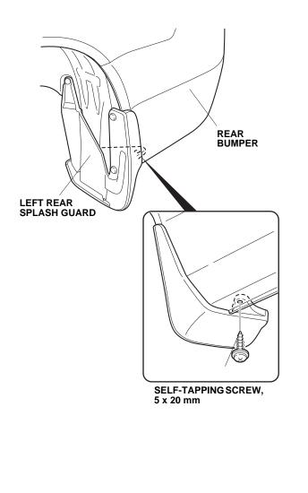
11. While holding the left rear splash guard against the rear bumper, tighten the four self-tapping screws in the order shown. Make sure there is no gap between the left rear splash guard and the vehicle. If there is, loosen the four self-tapping screws, adjust the splash guard to remove the gap, and retighten the screws.
