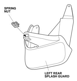
9. Install the left rear splash guard to the left rear inner fender with two 5 x 16 mm self-tapping screws and one self-tapping screw. Do not tighten the screws.
